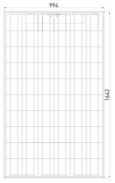
Tolerance of length and width dimensions is +/- 2 mm
