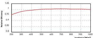
The typical relative change in module efficiency at an irradiance of 200W/m $^2$  in relation to 1000W/m $^2$  (both at 25 °C and AM 1.5 spectrum) is less than 6%
