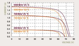
The typical relative change in module efficiency at an irradiance of 200 W/m² in relation to 1000 W/m² (both at 25  $^{\circ}C$  and AM 1.5 spectrum) is -7%.
